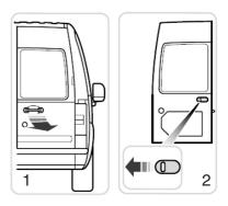
Open the left hand door second by squeezing the handle to unlatch the door and pulling it open.
